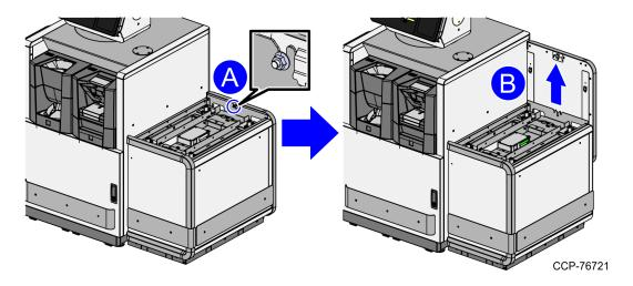
3. Remove two (2) nuts securing the Top Tray Pocket to the Rear Bagwell Panel, as shown in the image below.
