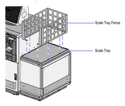
3. Secure the Scale Tray Fence on the Scale Tray using eight (8) screws, as shown in the image below.
