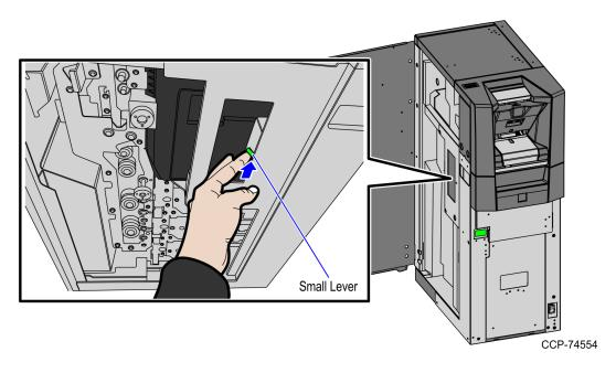
b. While holding the lever, push the green button on the front to open the Cassette Door.
