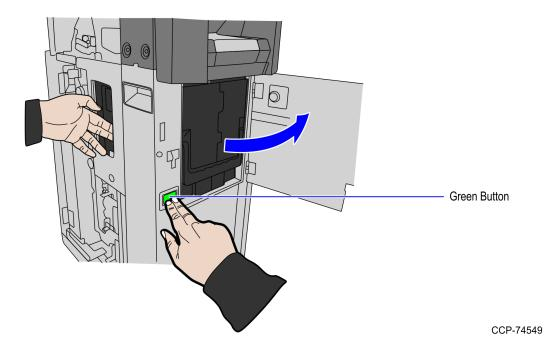
5. Remove the existing Note Cassette (Cashbox) or Note Interface Cassette (IFC) from the Note Recycler (Glory CI-10B) by pulling the handle as shown in the image below.
