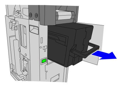
6. Insert the new Note Interface Cassette (IFC) by pushing it all the way in the Note Recycler (Glory CI-10B).
