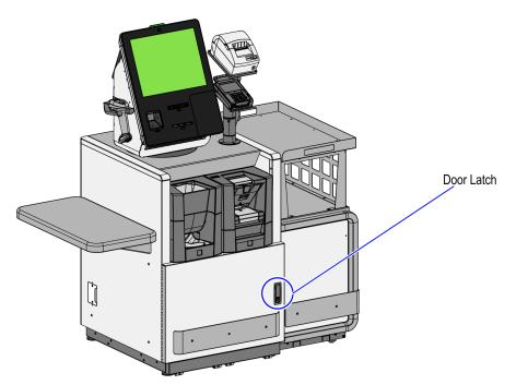
b. Remove key and then press the keylock to unlatch the door.
