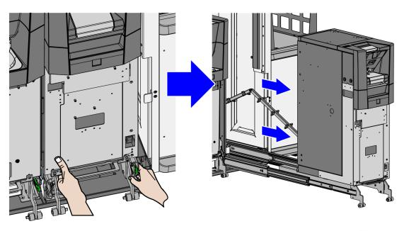
3. Insert key into lock on the left side of the Note Recycler (Glory CI-10B) and turn the key clockwise to open the side cover as shown in the image below.
