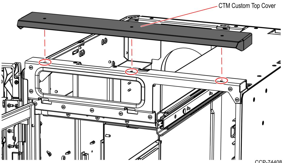
3. Secure the CTM Custom Top Cover with three M4 nuts using an M4 Nut Driver as shown in the image below.
