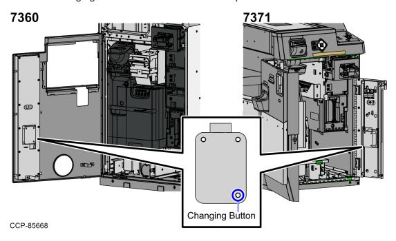
b. Insert a probe into the changing button hole and keep the changing button pressed.
