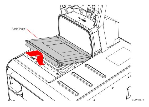
e. Install the Scale Plate on the Scanner.
