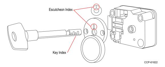
4. Insert the Change Key into the Change Key Hole on the back of the lock.
