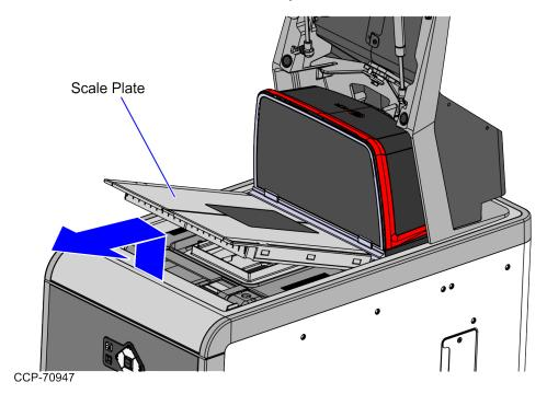
3. Remove the Scanner/Scale in the scanner bucket.
