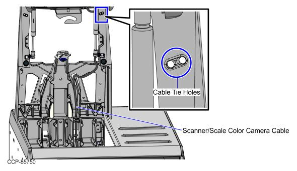
5. Insert excess cable into the space adjacent to the Tower Frame pole duct.
