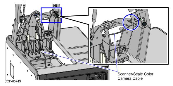
4. Secure the cables using a cable tie that is inserted through the holes on the Tower Frame.
