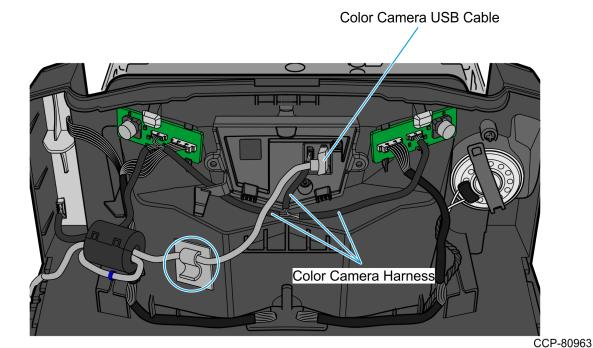
c. Route the other end of the Color Camera cable through the cable exit slot on the side of the tower, as shown in the image below.
