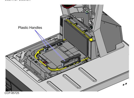
c. Push down the plastic handles on each side of the NCR 7896 Scanner/Scale.
