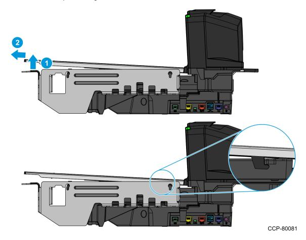
2. Hold the front edge and the top of the Top Plate to pull lift it off the Scanner/Scale.
