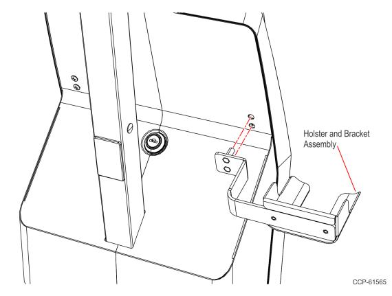
6. Secure the Holster and Bracket Assembly to the tower using two screws.
