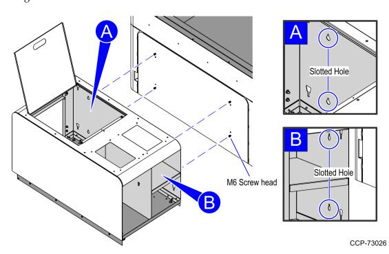
3. Insert and then tighten each M6 screw head into its corresponding hole slot as shown in the image below.
