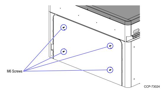
2. Align each M6 screw head with the slotted holes of the storage unit as shown in the image below.
