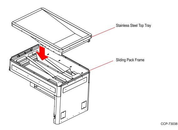
2. Secure the Stainless Steel Top Tray using ten M4 screws.
