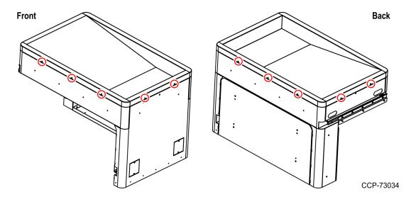
2. Lift and remove the Stainless Steel Top Tray from the Sliding Pack Frame.
