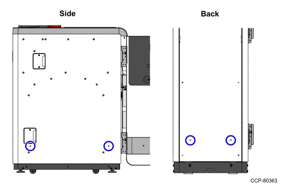
2. Attach the two (2) Side Lower Bumpers and secure each of them with two (2) Lock Nuts.
