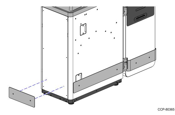
3. Install the Rear Lower Bumper and secure it with two (2) Lock Nuts.
