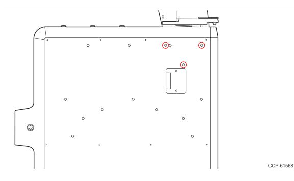
2. Align the Printer Shelf over the alignment screws and then slide the Shelf down onto the screws.
