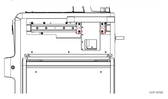
e. If the NCR Fastlane SelfServ<sup>TM</sup> Checkout (7360) unit's orientation is converted from self–checkout mode to assisted service mode, slightly lift the Shelf and slide it to the other end of the Slide Rail.
