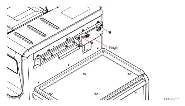
c. Align the Shelf Assembly key holes over the partially threaded screws and then slide the Shelf down onto the screws. Tighten the screws.
