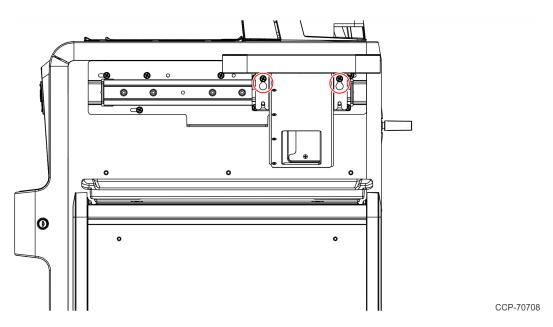
d. Install two (2) screws on the lower holes to secure the Shelf Assembly on the Hinge.
