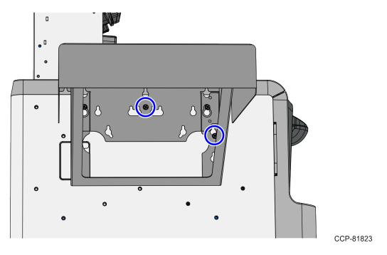
5. Tighten all four (4) M6 screws to secure the Basket Shelf to the unit.
