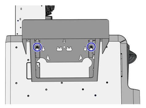
4. Insert two (2) M6 screws as shown in the image below.
