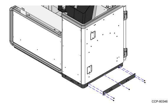
3. Attach the Bagwell End Skirt to the Bagwell using three (3) screws, as shown in the image below.
