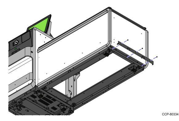
4. Attach two (2) 3-Bag Bagwell Skirts to the Bagwell using four (4) screws for each skirt, as shown in the image below.
