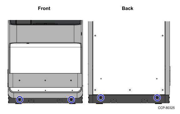
2. Attach the Side Skirts using ten (10) screws, as shown in the image below.
