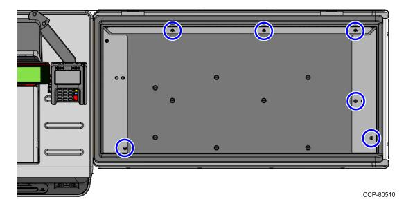
2. Lift and remove the fence from the Scale Tray.
