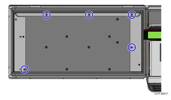
Note: Tighten the five (5) Acorn Nuts to secure the Side Fences to the Rear Fence.
