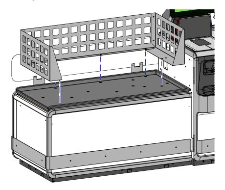
2. Secure the Scale Tray Fence on the Scale Tray using five (5) flat-head screws.
