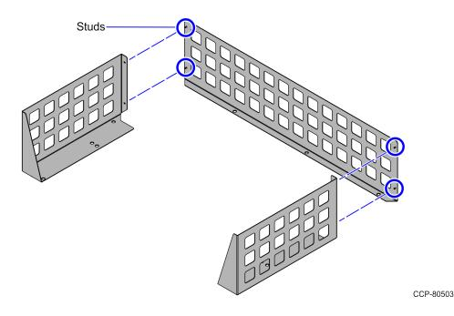
b. Loosely install four (4) Acorn Nuts on the studs.
