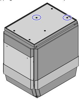
3. Secure the Bag Rack to the Scale Tray using two (2) screws.
