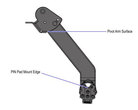
3. Fasten the PIN Pad Mount to the PIN Pad Arm using the Allen key.
