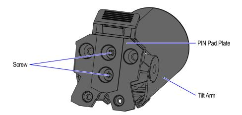
2. Remove the PIN Pad Plate and rotate it to 180°, as shown in the image below.
