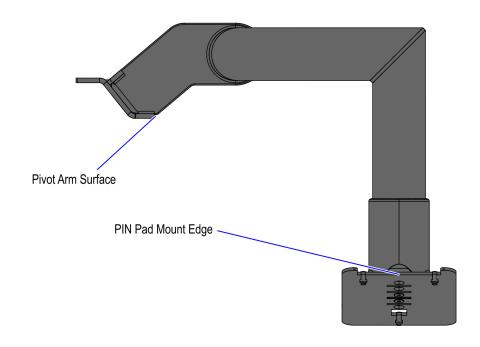
6. Fasten the PIN Pad Mount to the PIN Pad Arm using the Allen key.
