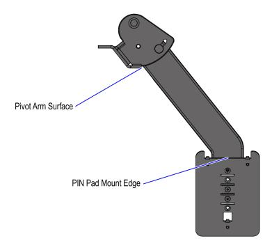
3. Fasten the PIN Pad Mount to the PIN Pad Arm using the Allen key.
