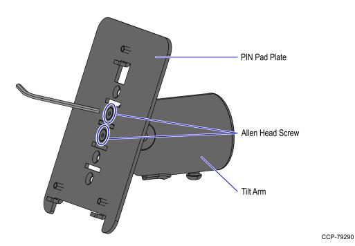
2. Remove the PIN Pad Plate and rotate it to 180°, as shown in the image below.
