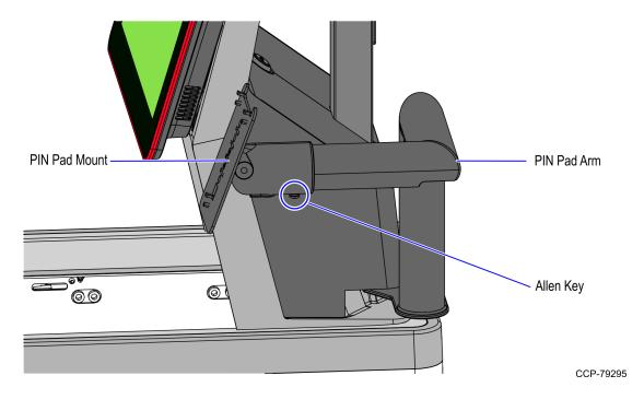
2. Remove the PIN Pad Mount from the PIN Pad Arm, as shown in the images below.
