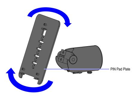
3. Install the PIN Pad Plate on the Tilt Arm using two (2) Allen head screws.
