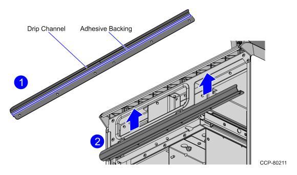
3. Press the Drip Channel firmly on the SelfServ Checkout Top Plate edge. Ensure that there are no air bubbles.
