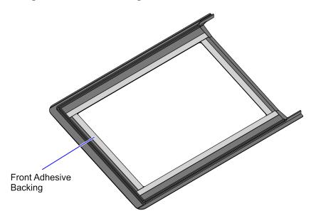
7. Align and attach the front edge of the Scanner Top Plate to the inner bottom wall of the Spill Protection Gasket, as shown in the image below.
