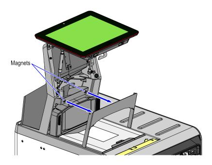
5. Remove the Scanner Top Plate from the Scanner.
