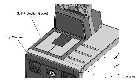
To install the Drip Channel, refer to *Installing Drip Channel* on the next page.
