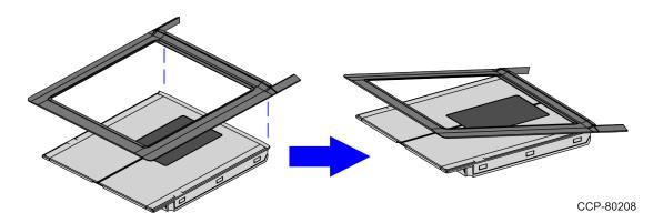
7. Remove the adhesive backing from the front and sides of the Spill Protection Gasket.
