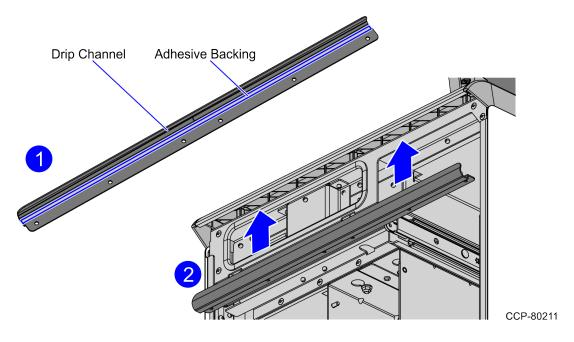
3. Press the Drip Channel firmly on the SelfServ Checkout Top Plate edge. Ensure that there are no air bubbles.
