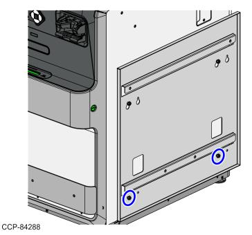
4. Tighten all four (4) screws to secure the Adapter Plate on the , as shown in the image below.
