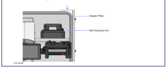
5. Align the holes on the End Panel of the Corner with the four (4) holes on the Adapter Plate and then secure using four (4) screws, as shown in the image below.
