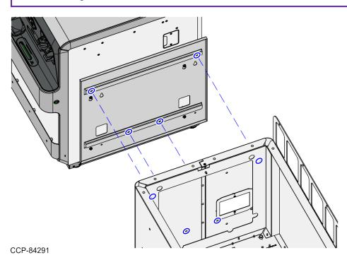
6. Install the Top Tray on the Corner Bagwell. Ensure that the captive screws on both ends of the Top Tray are aligned with the corresponding screw holes on the Bagwell.
