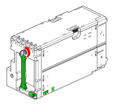
4. Hold the Notebox/Cashbox Module, slide the lid in the direction of arrows, and then lift it to open the Notebox (Cashbox) Module.
