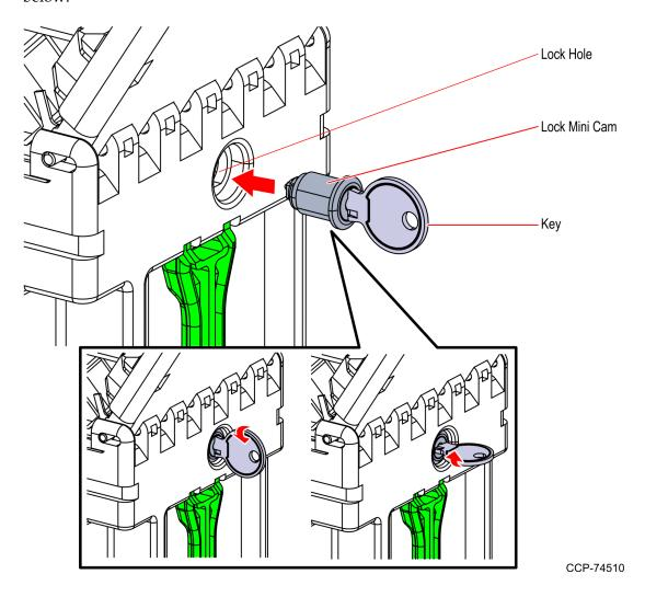
4. Secure the Lock Mini Cam using a retainer nut and torque the nut to 4 Nm or 35 in/lbs.
