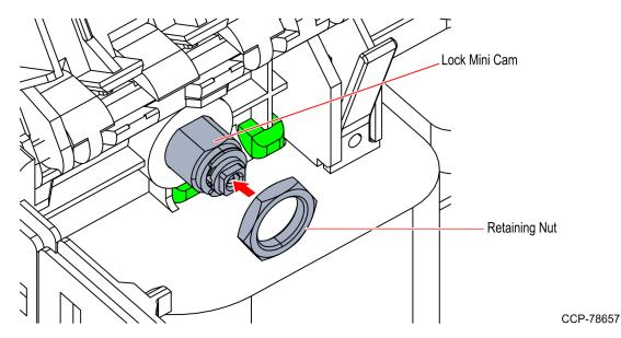
7. Remove the Lock Mini Cam from the lock hole of the Notebox (Cashbox), as shown in the image below.
