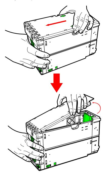
5. Detach the screw securing the Notebox (Cashbox) Cam to the Lock Mini Cam.
