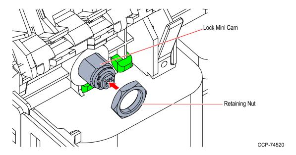
5. Attach the Notebox (Cashbox) Cam to the Lock Mini Cam using a screw. Torque the screw to 4 Nm or 35 in/lbs. Note the orientation of the cam in relation to the key position as shown in the image below.
