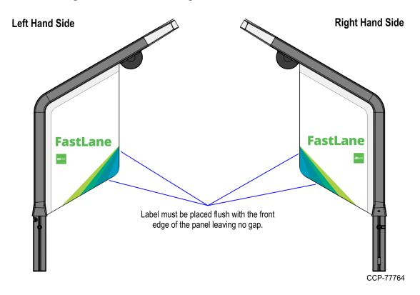
5. Hold half of the label in place while peeling off the protective film from the other half of the label and then attach the label on the Lane Light, as shown in the image below.
