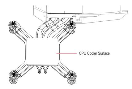
13. Install the CPU Cooler on the Motherboard.
