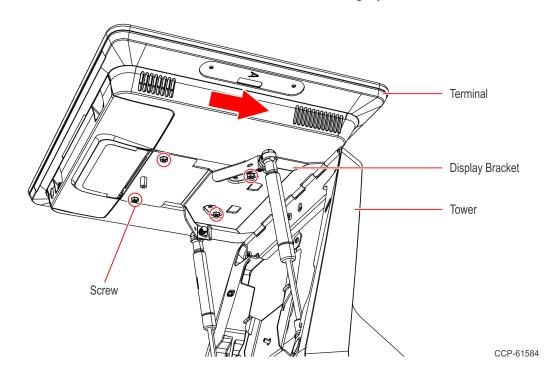
5. Lay the terminal face down on a flat surface.
