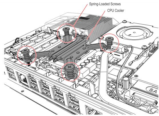
8. Remove the CPU Cooler.
