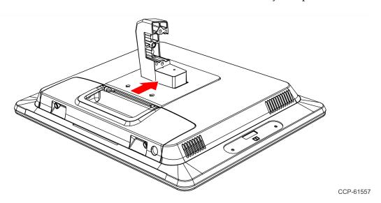
c. Secure the Plate and Brace Assembly to the Secondary Display using two screws.
