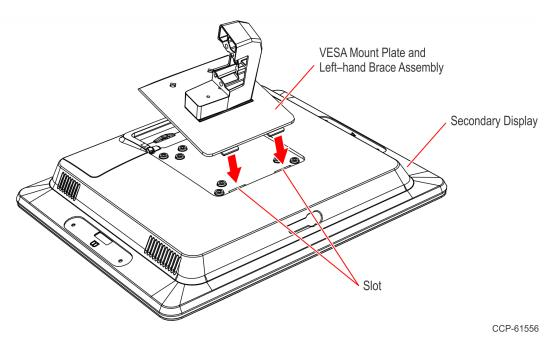
b. Slide the VESA Mount Plate and Left-hand Brace Assembly into place.
