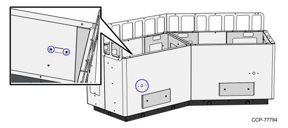
• Remove two (2) nuts to detach the Camera assembly from the Camera mounting hole.
