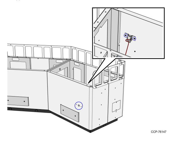
7. Route the cable to the SelfServ Checkout unit through the cable access holes of the Bagwells.
