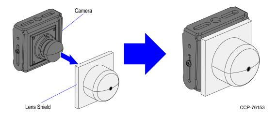
b. Insert the Camera into the Lens Shield Spacer hole, as shown in the image below.
