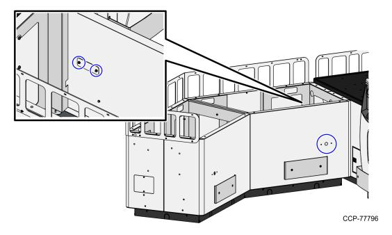
4. Route the cable to the SelfServ Checkout unit through the cable access holes of the Bagwells, as shown in the image below.
