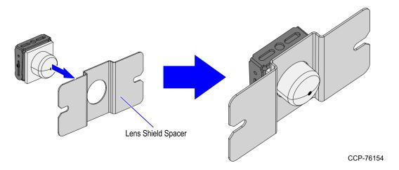
c. Position the Camera Bracket so that its screw slots are aligned with the screw slots of the Lens Shield Spacer.
