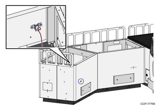
• Install the Camera blanking plate on the empty Camera mounting hole on the Bagwell wall.
