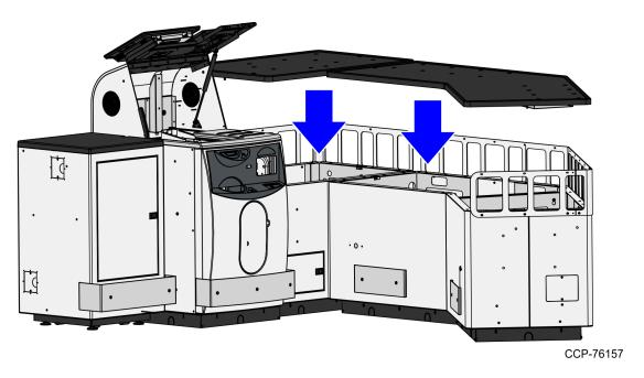
b. Push and turn the Service screws counterclockwise at approximately  $\frac{1}{4}$  turn to lock the top cover trays in place, as shown in the image below.
