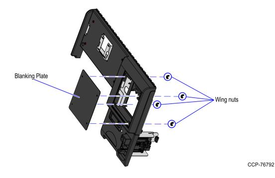
4. Align the Space Pole Adapter to the PIN Pad slot on the Upper Cabinet Door and then secure using four (4) wing nuts. Ensure that the orientation of the Space Pole Adapter is the same with the image shown below.
