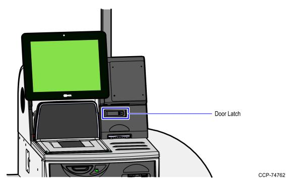
2. Remove the key and then press the keylock to unlatch the door.
