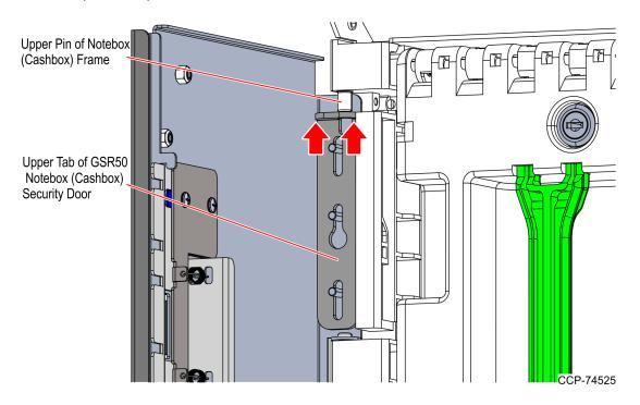
4. Secure the upper tab of the Security Door using three (3) hex nuts and then torque the nuts to 4 Nm or 35 in/lbs.
