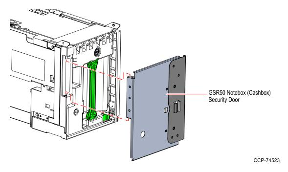
2. Place the lower tab of the GSR50 Notebox (Cashbox) Security Door over the lower pin of Notebox (Cashbox) frame.
