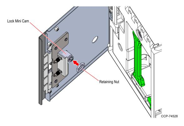
7. Attach the Security Door Cam to the Lock Mini Cam in a vertical position using a screw and torque the screw to 4 Nm or 35 in/lbs. Ensure that the key can rotate to 1/4 turn clockwise.
