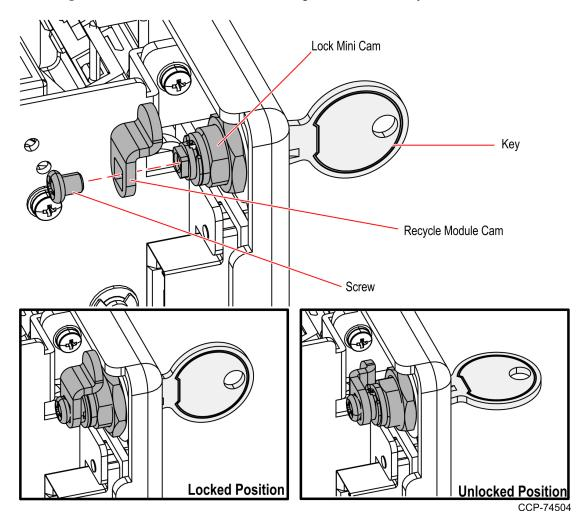
5. Apply an adhesive (Loctite #242) to the cam screw to secure the cam in place. To install the Notebox (Cashbox) Security Door, refer to *Installing GSR50 Notebox* (Cashbox) Security Door on the next page.
