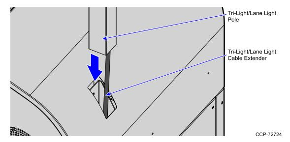
3. Secure the pole to the Upper Cabinet using two screws.
