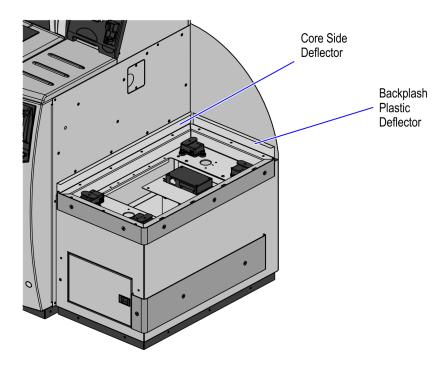
7. Attach the Scale Tray to the Bagwell using four (4) flat-head screws.
