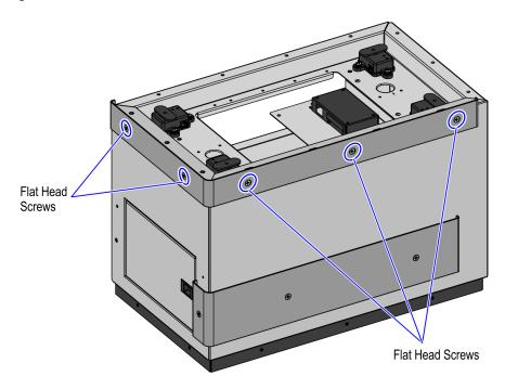
c. Attach the Backsplash to the Bagwell frame using four (4) flat-head screws.
