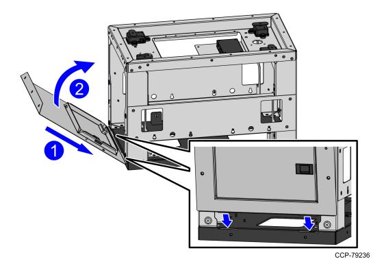
b. Secure the Front Panel to the Bagwell frame using two (2) nuts, as shown in the image below.
