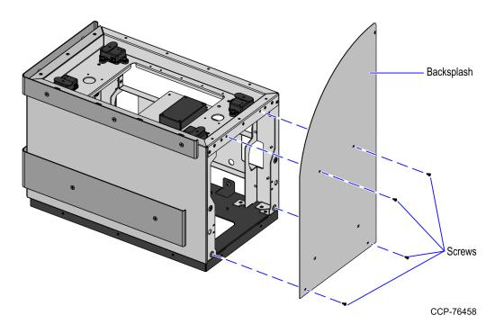
d. Secure the Backsplash to the Core using one (1) screw.
