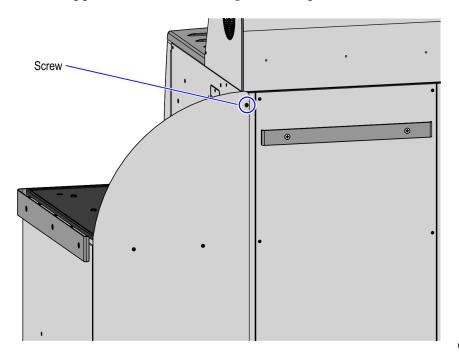
c. Detach the Backsplash from the Bagwell by removing four (4) flat-head screws.
