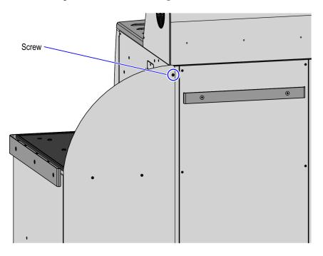
e. Attach the lower-rear bumper to the Bagwell using two (2) flat-head screws.
