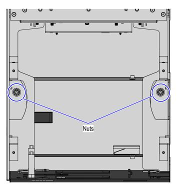
b. Pull down the Front Panel and then pull out to disengage from the slots in the Bagwell frame base, as shown in the image below.
