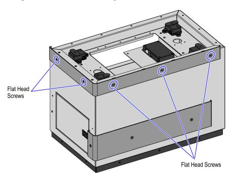
e. Detach the wrap-around side bumper by removing three (3) flat-head screws and spacers, as shown in the image below.
