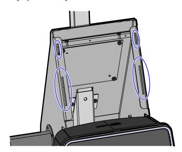
10. Secure the Terminal Display to the Tower Frame using two (2) screws.
