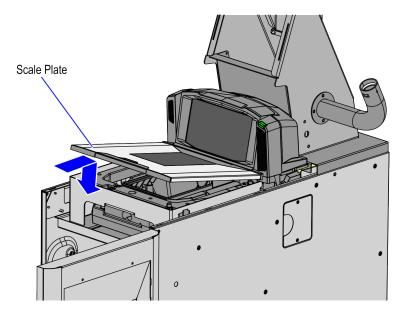
d. Install the Scanner Top by sliding it toward the Tower Frame.
