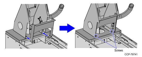
7. Install the Adapter Plate on the Scanner Bucket, as shown in the image below.
