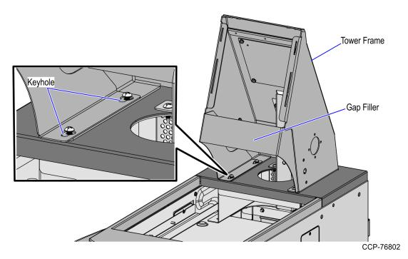
5. Push the Gap Filler toward the back and then tighten the screws, as shown in the image below.
