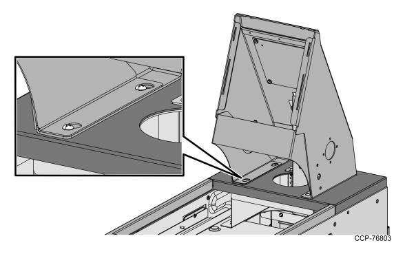
6. Install the Supervisor Switch including the Supervisor Switch Bracket and P-Loop using two (2) Hex nuts.
