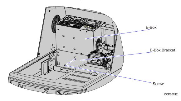
3. Remove the E–Box with the Cable Guide still attached.
