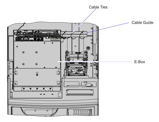
8. Position the E–Box to its working position.
