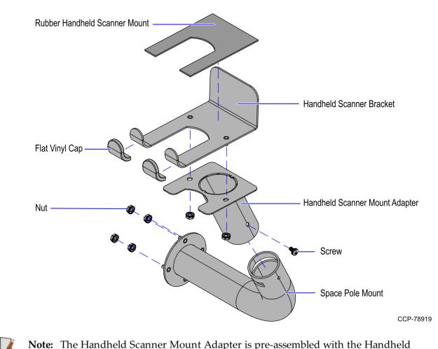
**Note:** The Handheld Scanner Mount Adapter is pre-assembled with the Handheld Scanner Bracket, Flat Vinyl Cap, and Rubber Handheld Scanner Mount prior to shipment.
