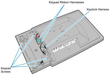
3. Remove the Keypad Bezel from the Front Bezel.
