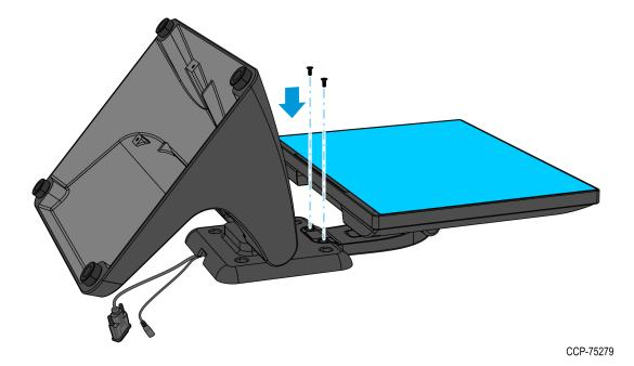
4. Position the stand onto the back of the display, and then secure with four M4x10 screws.
