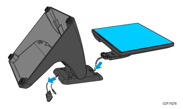
3. Position the neck of the Customer Display onto the display holder compartment, and then secure with two M4x6.5 screws.
