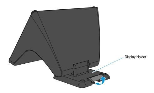
2. Remove the compartment cover on the neck of the Customer Display.
