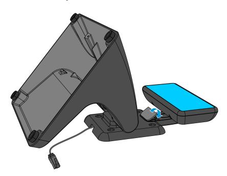
6. Position the stand onto the back of the display, and then secure with four M4x10 screws.
