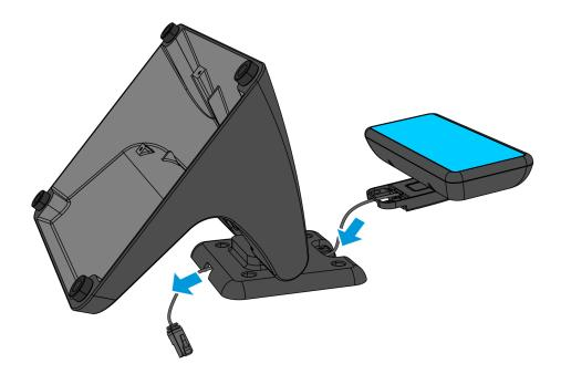
4. Position the neck of the Customer Display onto the display holder compartment, and then secure with two M4x6.5 screws.
