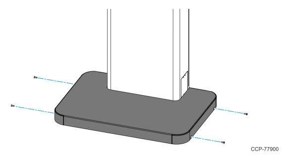
2. Align the four mounting holes on the pedestal base with the four mounting holes on the baseplate.
