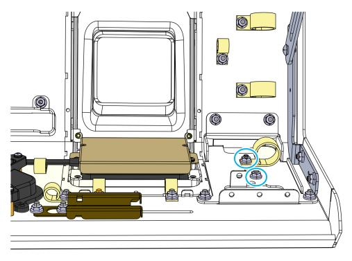
4. Connect the MSR USB cable to the MSR device through the cable access hole for the USB connector, and then use a cable tie to secure it to the metal bracket just above the connector.
