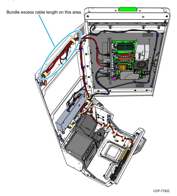
2. Secure the cable with cable ties and p-loops along its route.
