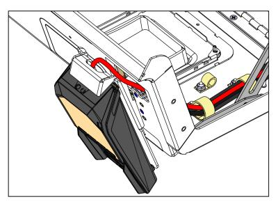
4. Install the PIN Pad Assembly onto the kiosk.
