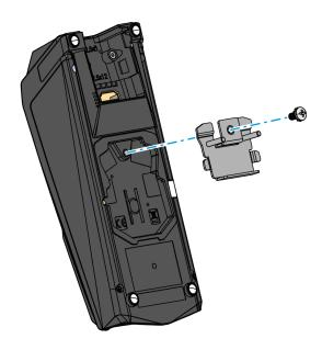
2. Install the PIN Pad on the mounting bracket.
