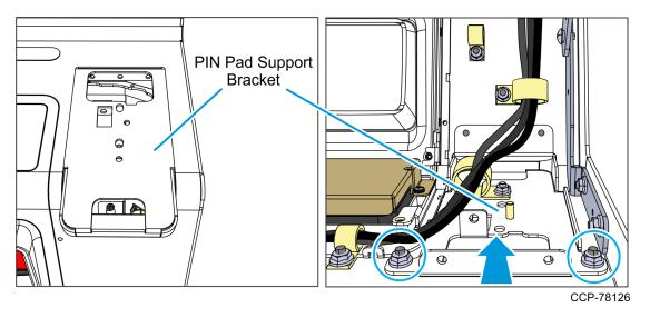
2. Tighten the two upper nuts and install the two bottom nuts, and then secure the cable bundle into the p-loop.
