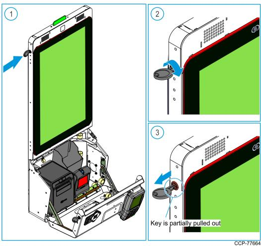
b. While the key and the cam lock are at the OPEN position, grip the left edge of the Upper Module Door and pull the door forward.
