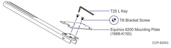
Install the payment device on the Equinox 6200 Mounting Plate using the screws included in 1668-K150. Use the T10 Torx L Key (included in 1668-K150) to tighten the screws.
