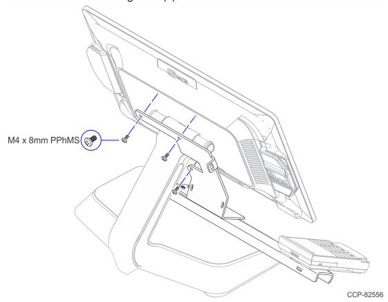
CX7 with 7772-K320 (Bracket, Wall Mount, Integrated I/O) — Install the 7772-K320 Wall Mount and Side of Monitor Support VESA Bracket on the back of the NCR CX7 POS using a Spacer and four (4) M4 x 10mm PPhMS.
