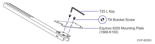
3. Install the payment device on the Equinox 6200 Mounting Plate using the screws included in 1668-K150. Use the T10 Torx L Key (included in 1668-K150) to tighten the screws.
