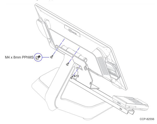
CX7 with 7772-K320 (Bracket, Wall Mount, Integrated I/O) — Install the 7772-K320
