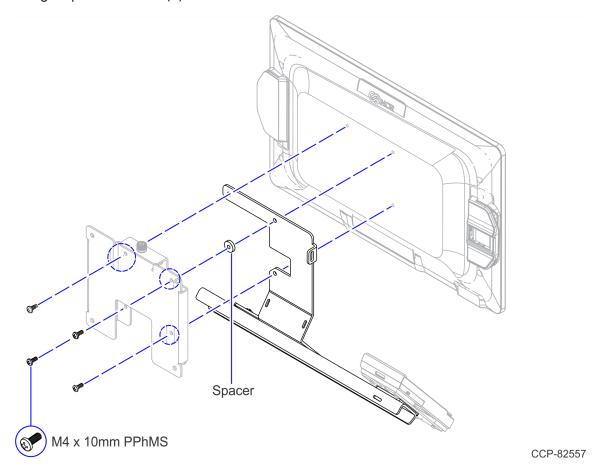
CX7 with 7772-K325 (Bracket, Wall Mount, Power Supply, Integrated I/O) — Install the 7772-K325 Wall Mount and Side of Monitor Support VESA Bracket on the back of the NCR CX7 POS using a Spacer and four (4) M4 x 10mm PPhMS.
