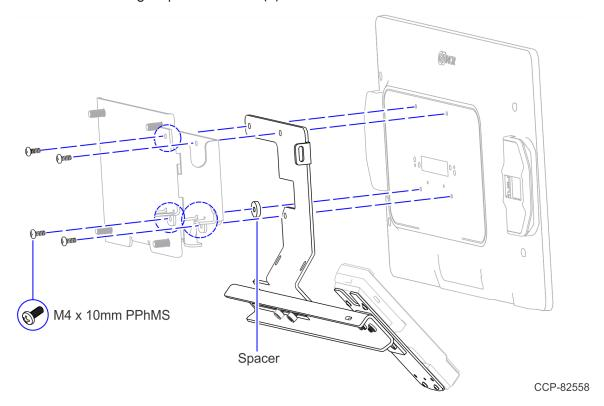
6. Adjust the payment device position by sliding the CX7 Side of Monitor Mounting Bracket left or right. Once desired position is reached, tighten the four (4) M5 x 0.8mm SHCS as shown below.
