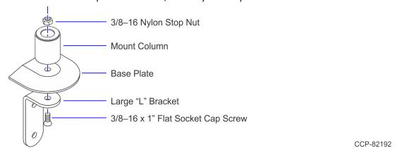
b. Install the assembled Mount as shown using two (2) screws. Use hardware appropriate for the surface being mounted on.
