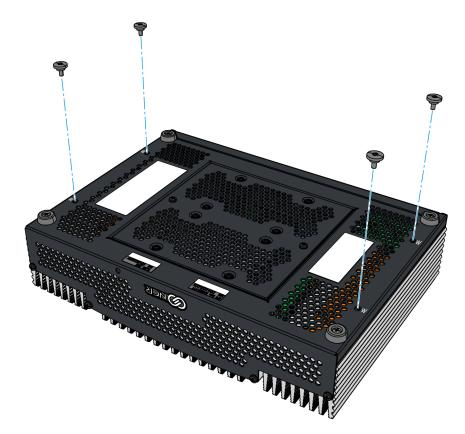
5. Position the N4000 beside the bracket, mount the four Step Pan Head Flat Screws onto their slots on the bracket, and slide the N4000 downward to lock it in place.
