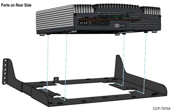
5. On the rear side, secure the N4000 with the included security screw.
