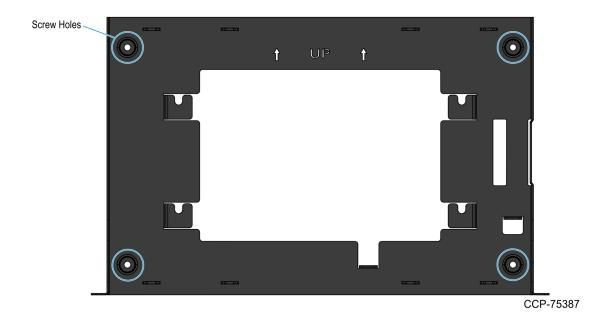
2. Use the toggle bolts to secure the Mount Bracket to the wall.
