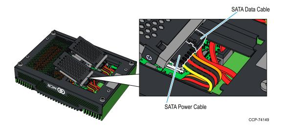
b. Slide in the bracket so that the bottom cover feet are on top of the bracket feet, and then push down the SSD bracket.
