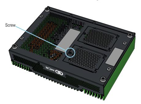
4. Using a Phillips screwdriver, install the four screws on the front panel.
