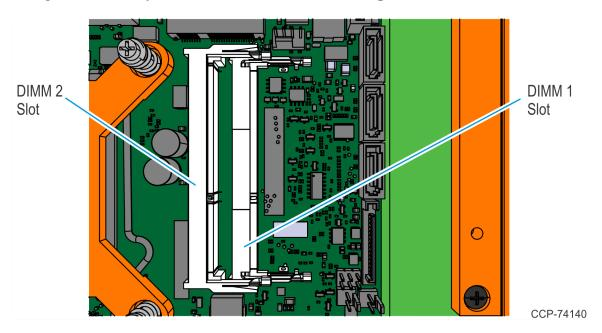
! Important: All memory features containing one memory module should be installed into the lower socket (DIMM 1 Slot). Any memory upgrade that requires adding an additional memory module should be installed in the upper socket (DIMM 2 Slot).
