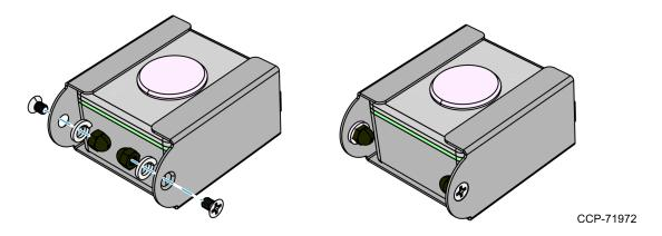
3. Connect the Small Single Button Box to the Button Controller Box using the RJ11 cable.
